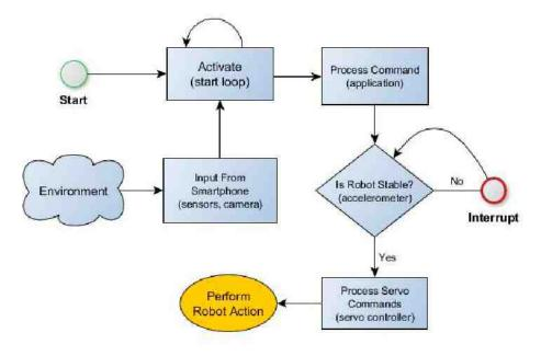
Figure 3,7: Execution process for robot application.
