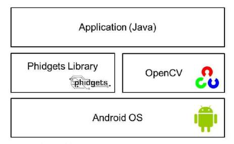
Figure 4.3: Software stack for the robot platform.
