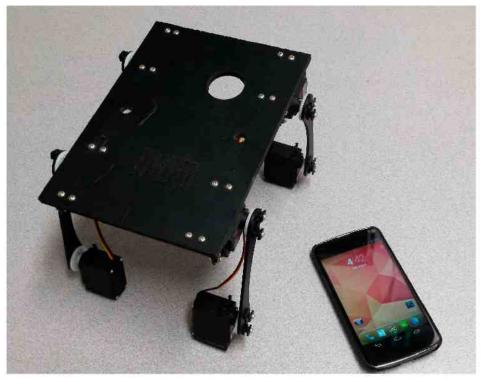
(a) Assembled base of the robot.
