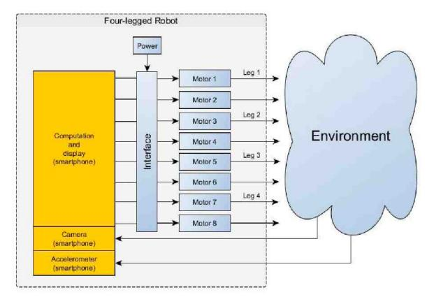
Figure 3.5: System block diagram for the robot platform.
