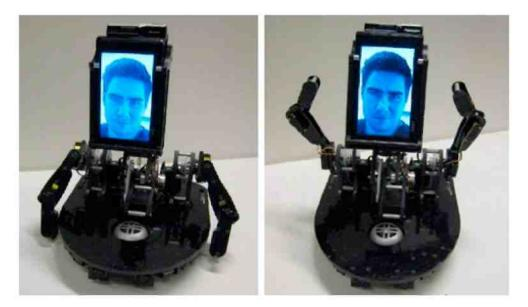
Figure 2.3: MeBot mimics the head and arm movements of user.
