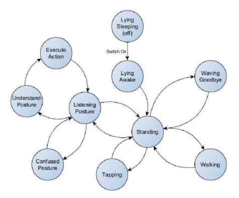
Figure 3.6: State transition diagram for robot application.
