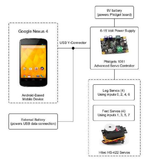
Figure 4.2: Schematic showing the connections for each robot component.
