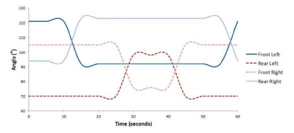
(b) Angles ploted for all four robot legs as it walks. Two legs diagonally opposite from each other alternate movement giving the robot a brisk walk with stability.
