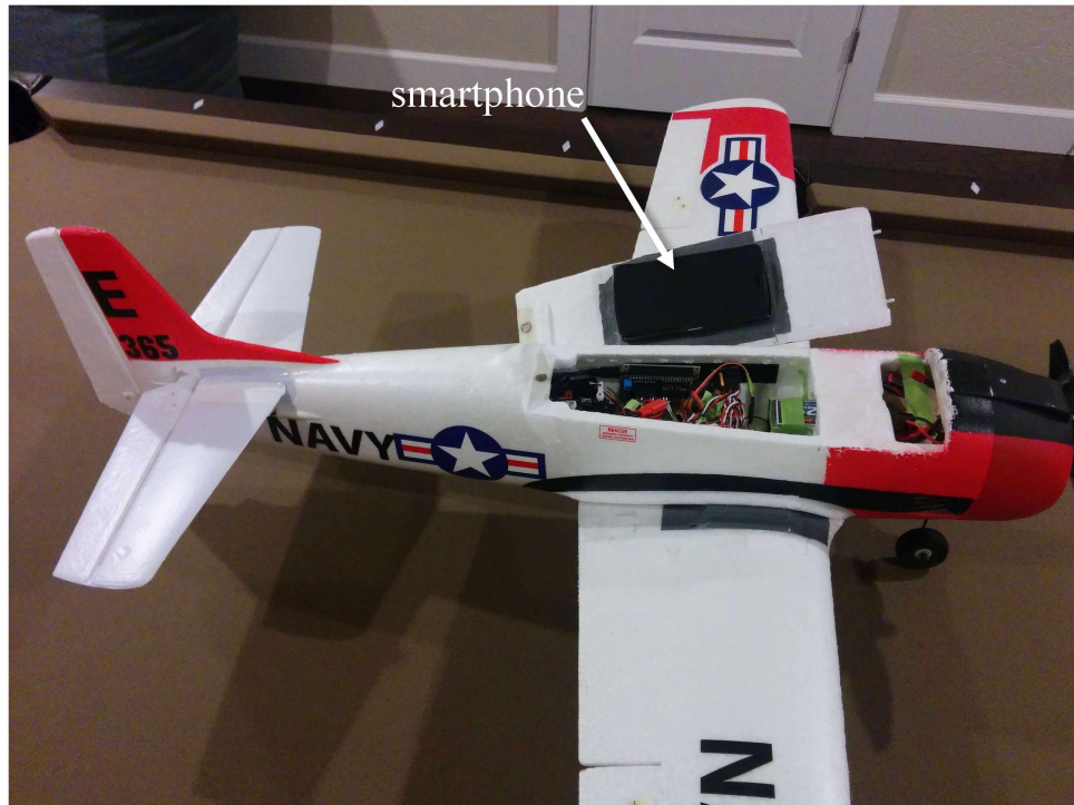
Figure 24. UAS experimental platform (Parkzone T-28 RC airplane)
