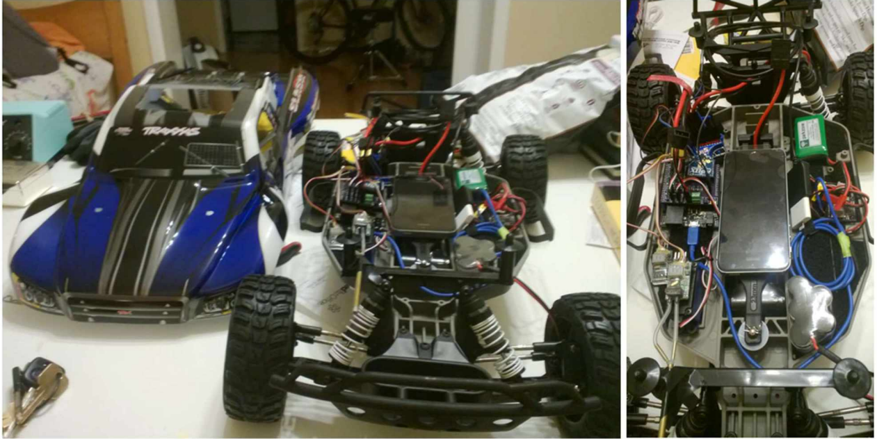
Figure 22. Unmanned ground vehicle with smartphone controller
